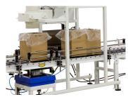
**PLATFORM SCALE** Platform scale allows final packaging container to be tared and filled into directly.
